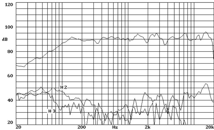
Note: on axis frequency response measured with loudspeaker standing on infinite baffle in anechoic chamber, 1w @ 1m. Crossover frequency set at 3kHz@12dB/oct.
